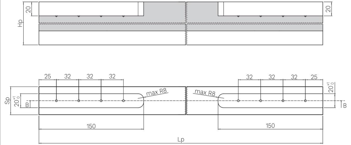
Hp = door leaf height (mm) - Lp = door leaf width (mm) - Lb = track length (mm) - Sp = door leaf thickness (mm)
